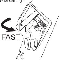
Figure 27. Throttle Lever (Fast Position)
